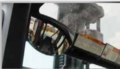
Dual panoramic interior rear view mirrors standard Dual external side view mirrors standard Optional pedestrian camera and monitor
