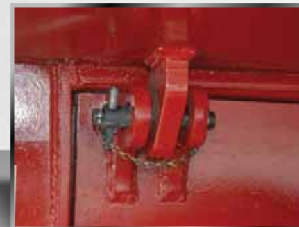
The 4 removable pins and 4 lifting eyes make it easy to remove and install the counterweight.* *Caution should always be taken when moving any load. Please refer to manual for proper procedures before removing the counterweight.
