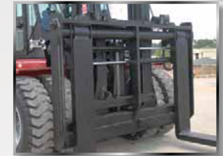
The pin-mounted forks are hammer forged from heat treated steel with increased thickness in critical heel sections. The forks are fully adjustable from full width of carriage to +/-2-in. Lengths and widths vary depending on your particular needs and model type.
