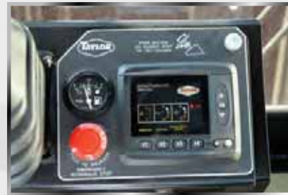
Easy to understand diagnostic display. TICS (Taylor Integrated Control System) using CANbus technology is standard on the TX-550RC
