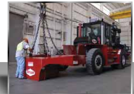
The 4 removable pins and 4 lifting eyes make it easy to remove and install the counterweight.* *Caution should always be taken when moving any load. Please refer to manual for proper procedures before removing the counterweight.
