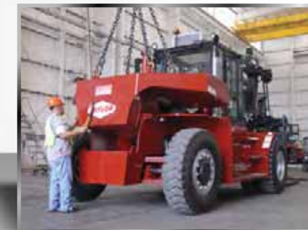
The 4 removable pins and 4 lifting eyes make it easy to remove and install the counterweight.* *Caution should always be taken when moving any load. Please refer to manual for proper procedures before removing the counterweight.
