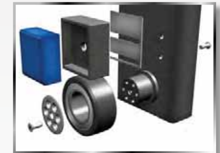
The mast and carriage main rollers are common and use Timken® tapered roller bearings. Chain rollers use sealed ball bearings. Common, cast nylon, side thrust pads are adjustable to compensate for wear.
