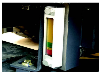
Autolube is a standard feature on the Taylor T-1023. All pressure taps and site gauges are easily accessible. Fluid drains provide environmentally friendly drainage capability and are grouped together for convenient serviceability.
