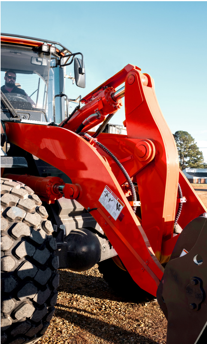
The Taylor T-1025 features optimized Z-Bar geometry that positions the bucket closer to the tires, achieving high bucket breakout forces with maximum rollback. The option of hydraulic quick coupler attachment adds versatility to Z-Bar machines, allowing use of multiple tools to suit the job-site needs.
