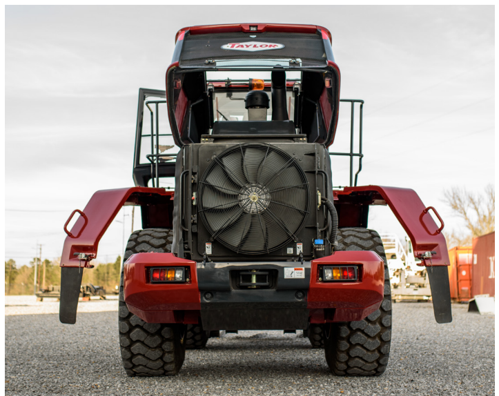
The rear full fenders swing out for easy access to the engine compartment. The electrically actuated, wide opening fiberglass hood of the Taylor T-1035 gives you easy access to the engine and its easy-to-reach service points. The radiator also swings out for ease of service.
