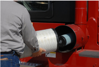
Donaldson Air Cleaner with Safety Element (Standard)
