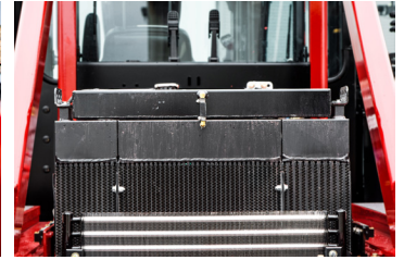
3-Section Bolted Radiator (Each section can be serviced separately)
