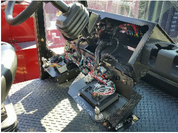
Flip-down Dash with Color/Number Coded Wiring (Standard)
