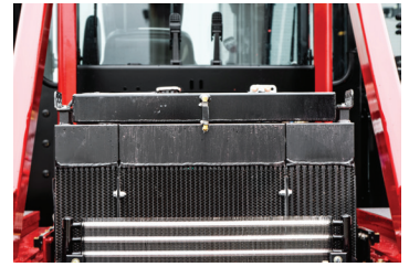
3-Section Bolted Radiator (Each section can be serviced separately)
