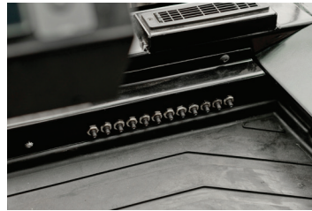
Heavy Duty Circuit Breakers/Reset Switches (Standard)
