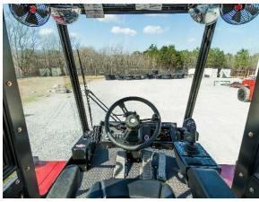
Climate Controlled 2-door Cab - All Steel - Heat, A/C & Defrost (Standard)
