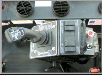
A simple joystick is far easier to operate than multiple levers.
