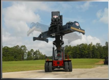
Hydraulic allow 95° of CCW rotation and 185° of CW rotation for superior maneuverability.
