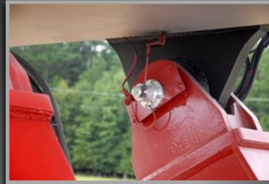
Electronic boom angle sensor mounted directly to the tower and boom gives a more reliable and precise angle reading.
