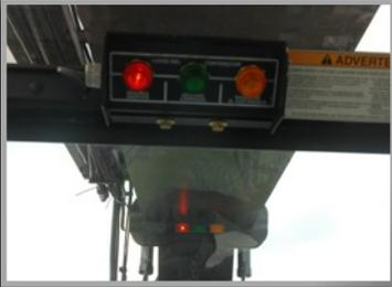
In cab and on boom viewing of indicator lights .
