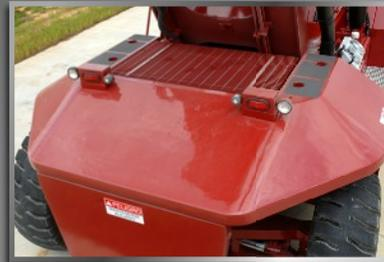
For the safety of on-the-ground workers, the TS-9972 has added rear facing camera, taillights, work lights, and motion alarm to the sloping counterweight.
