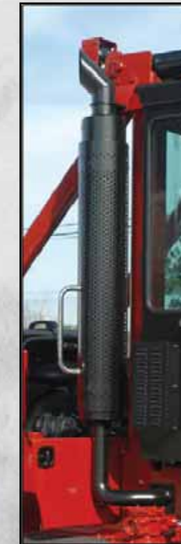
Features an outboard mounted, heat shielded, muffler with vertical stack for improved visibility and noise control.
