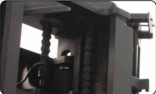
Lift chains are hidden inside mast rails
