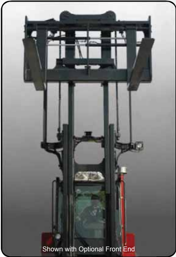
Two-stage telescopic mast Nested channels Lift cylinders behind rails
