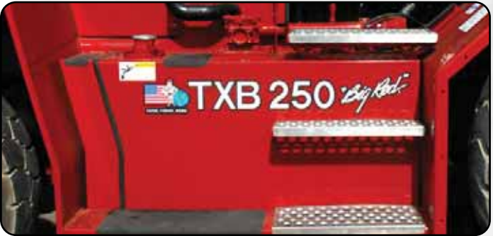
Bolt-on tanks on all TX, TXH and TXB Series trucks.
