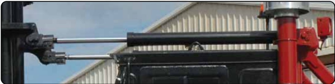
Overhead tilt cylinders Adjustable rod ends Greaseable self-aligning spherical bearings Better mast stabilization
