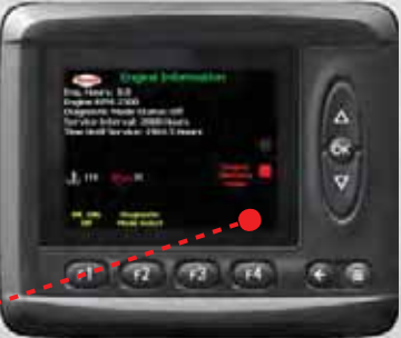
Electronic diagnostics with fault code history for fast problem identification.
