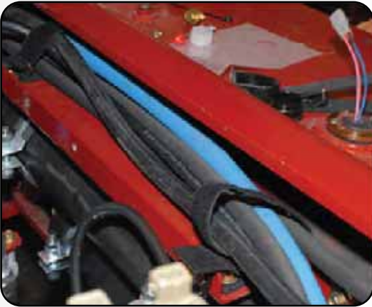
Frame Channels For clean and protected routing of wiring and hoses
