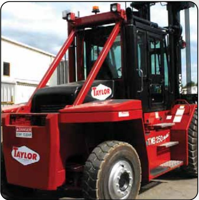
Counterweight sections are sloped to provide increased visibility for the operator
