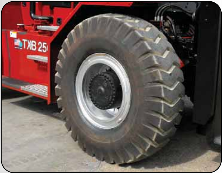
Heavy-duty bolted planetary drive axle 3 planetary pin, force-cooled wet disc brakes Hydraulic activated, brake saver system does not allow operator to drive through parking brakes Din type rim mounting Internal, force-cooled hydraulic actuated service brakes Wet disc brake oil and hydraulic oil are cooled by hydraulic cooler
