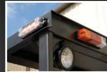
Slim fitting strobe lights, brake/signal lights, and work lights for increased safety and visibility.
