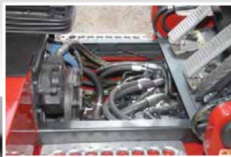
Simple, removable floor plate further adds to the access of the drivetrain.
