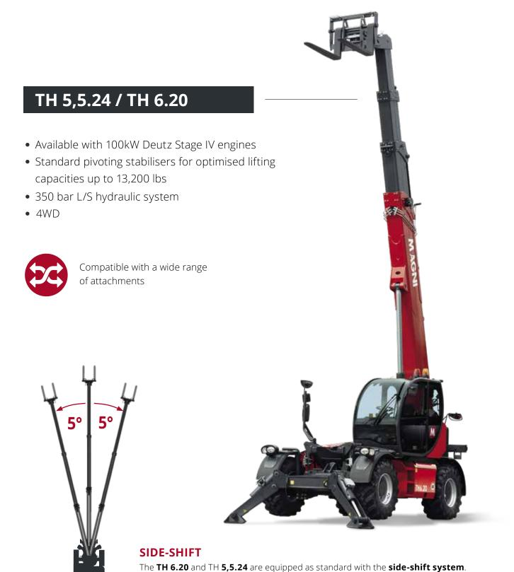
It allows for lateral movement of the rear part of the chassis and the boom, around the longitudinal axis of the machine, correcting the position of the load without moving the unit. This system allows for a +/-5° shift which corresponds to a +/- 5 ft movement when
